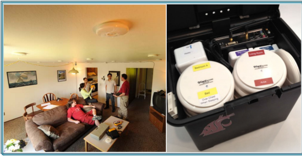
Fig. 1. (Left) Motion/light sensors and door/temperature sensors are installed in a smart home; (right) the SHiB kit includes sensors, computer, and networking equipment.
